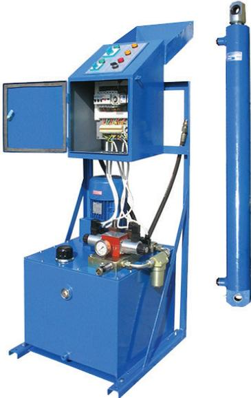
Actuator 90-0300 is applied oscillating motion with fixed amplitude according to the cylinder stroke. Movement of the cylinder rod can be continual or with a pause at the end position. Changing direction of the movement carried out without proximity switches so the device is insensitive of the dust and humidity.
