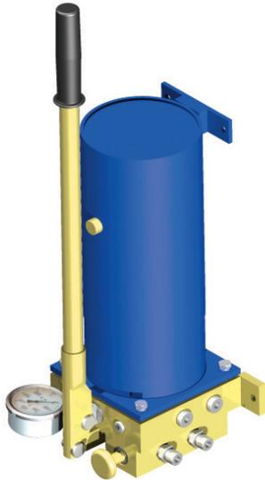
Hand pump operates in combination with double acting cylinder. High-pressure hose of 3 m length is included in delivery. Cylinder has to be ordered separately. Robust design, high precisely part treatment, high quality seals provide long time exploitation of the hand pump. Delivered pump is filled with oil and ready for use. Before use release the breather screw and retight the unloading handle.
